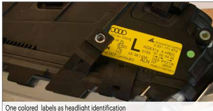
One colored labels as headlight identification
