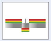
The cutting tools always consist of a tamp and a counter-cutting plate. A typical example is the die-cutting of holes into paper for pinfeed or filing applications.
