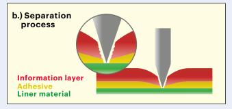
cutting surface (liner material) should remain intact.
