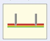
The severing / die-cutting of the material is done in two steps. In the compression phase, the composite material is compressed. Then the cutting blade reaches the solid surface; the material is now severed. The separation process is dependent on the material to be cut and on the cutting angle used. The soft material components are compressed.
